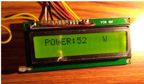
Figure 6: LCD display showing energy usage
